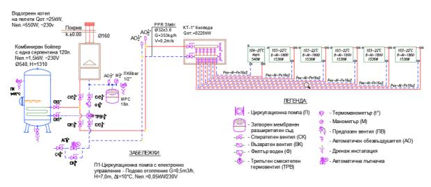
Figure 1.3. Pipe diagram of equipment, safety and control valves
