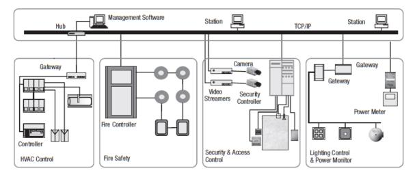
Figure 2.3. Integrated intelligent building system
