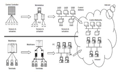
Figure 2.1. Progress of computerized automation systems
