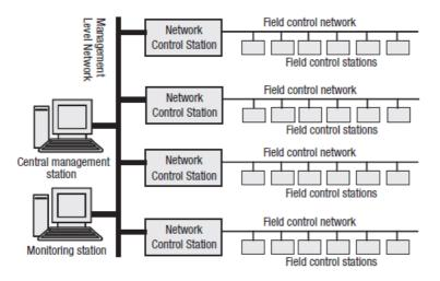
Figure 2.2. Typical BAS network architecture
